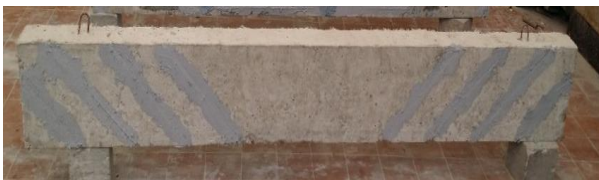
Fig. 6 Strengthening preparation of NSM Inclined GFRP bar
