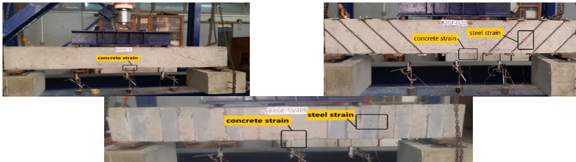
Fig. 10(b) the positions of the electrical strain gauges
